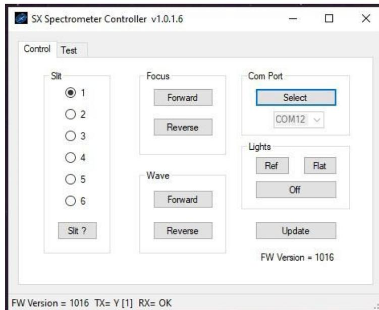
The spectrograph is automatically started with the slit set to the highest resolution position (Number 1, 20 microns wide x 1mm high). This is usually the best setting for general purpose use, but may be changed by selecting another option on the 'radio buttons' at the left side of the software menu.
