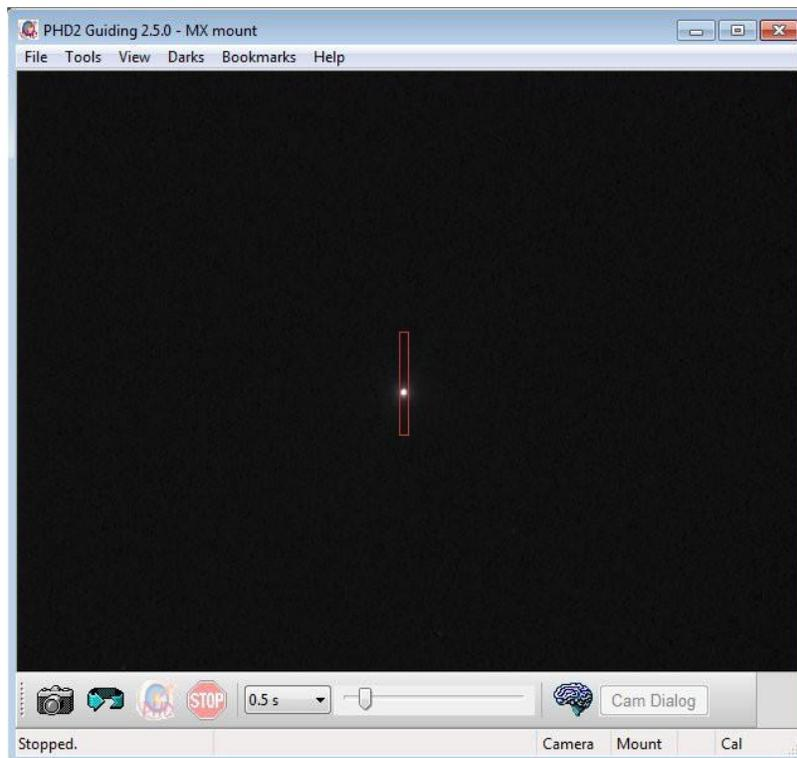
If you have a test target in mind, slew to this object and find a good bright guide star in the field, otherwise find any bright star to calibrate PHD2. Use the mouse to click on the guide star and then click on the 'target' icon in PHD2. A green guide box and cursor will appear and centre on the star, PHD2 will then run a calibration sequence to determine the optimum guiding parameters. Once completed, PHD2 will begin to guide on the selected star.
