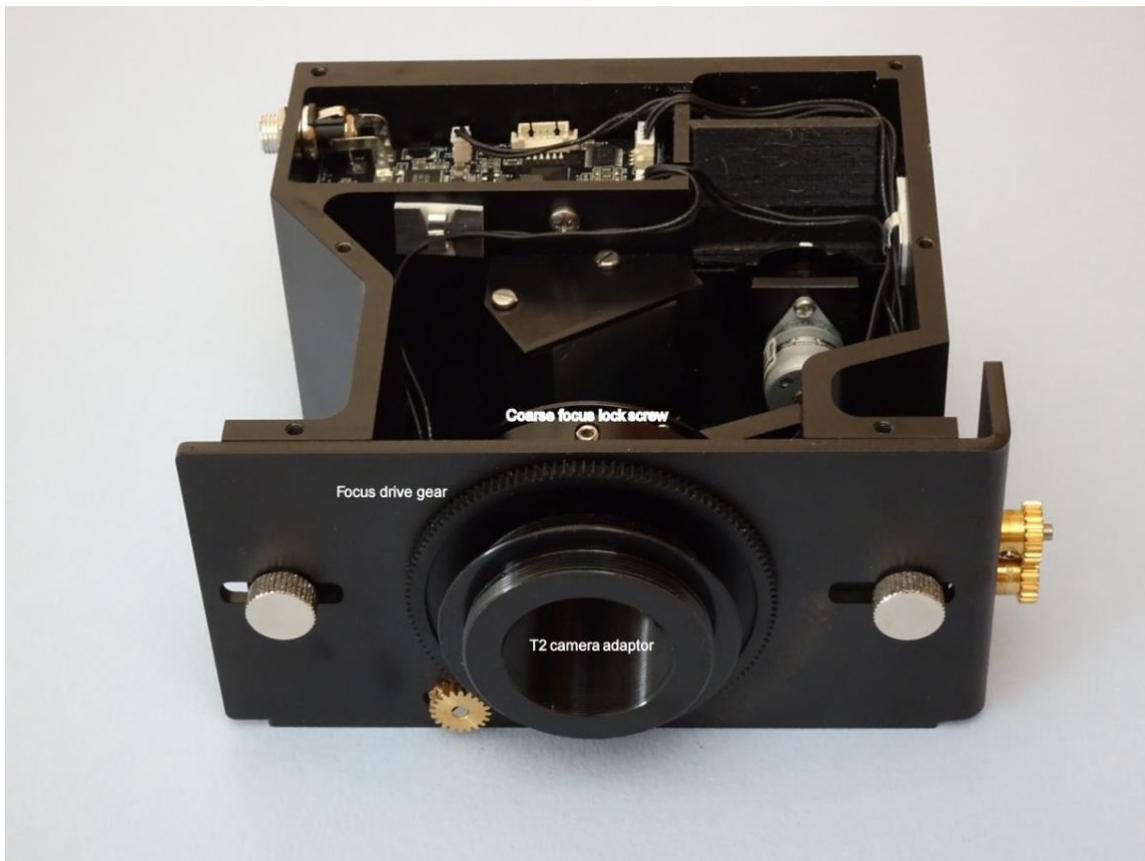
The camera is attached via the male T2 thread on the output adaptor, as shown below:
