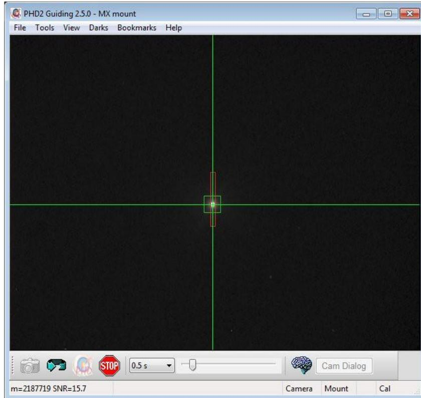
You can now see if the spectrograph will give a spectrum from an object within the slit cursor of PHD. To test this, switch off guiding in PHD2, set PHD2 to looping images, and then slew a bright star into the spectrograph slit cursor box. The slewing can be done by using the 'Manual guide' option in PHD2, or by operating your telescope controls. Centre the star in the slit cursor and then select it as the guide star, so that PHD2 keeps it in position.
