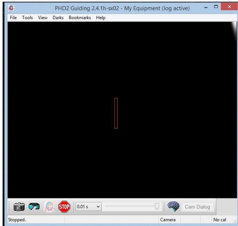
You should now be able to start PHD2 on an imaging cycle (use the 'Loop' symbol to start it), and set up the focus on a guide star. Point your 'scope at a dense star field with many bright stars to make this job as easy as possible - open clusters like M44 are good targets. With any luck, you will be able to see several stars when using a 1 or 2 second exposure, and be able to refine the focus until the stars are sharply defined.
