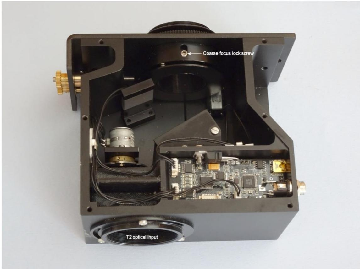
The T2 thread is part of a removable barrel that is normally locked into a fine-focus sleeve by an M4 setscrew (accessible when the box cover is removed). The fine focus sleeve is itself driven by the large ring gear, which is seen surrounding the T2 adaptor. One rotation of this ring, moves the camera in or out by 0.75 mm, and permits the accurate focusing of the spectrum onto the camera sensor.
