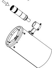
remove the dust cover and Loosen the thumbscrews on the end of the focuser adapter.
