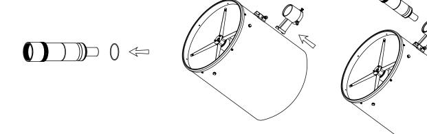
remove the dust cover and Loosen the thumbscrews on the end of the focuser adapter.
