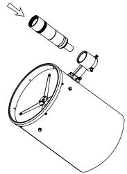
remove the dust cover and Loosen the thumbscrews on the end of the focuser adapter.
