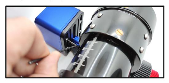
Once you have installed the motor kit, you don't need the drawtube brake, as the motor locks the shaft. (don't try to turn the knob by hand as the motor kit has a gearbox and you may damage it).
