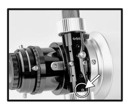
Remove telescope focuser's coarse knob . (Avoid to install the motor kit to 1:10 fine focus knob as the motor has very high step resolution).
