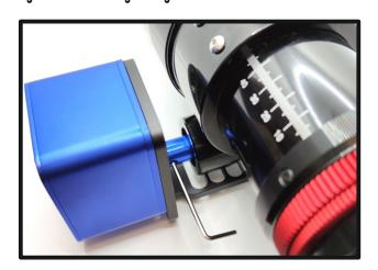
Use your 2.5mm Allen key and tight well the 4 x Allen bolts to secure the motor on the bracket.
