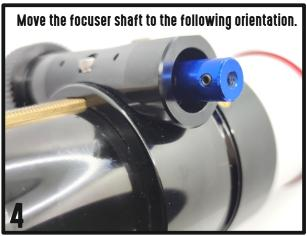
Attach the motor to the focuser and join the coupler with motor shaft. (do not tie yet the set screws of the motor coupler).
