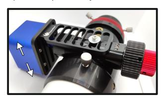
Use your 2mm Allen key and tight well the set screws on the motor side.
